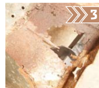
3 Rotten footwells – typical of many older Land Rovers. If the top half is still solid, these can be repaired, otherwise a complete new footwell is required. This one has already been patched at one stage...
