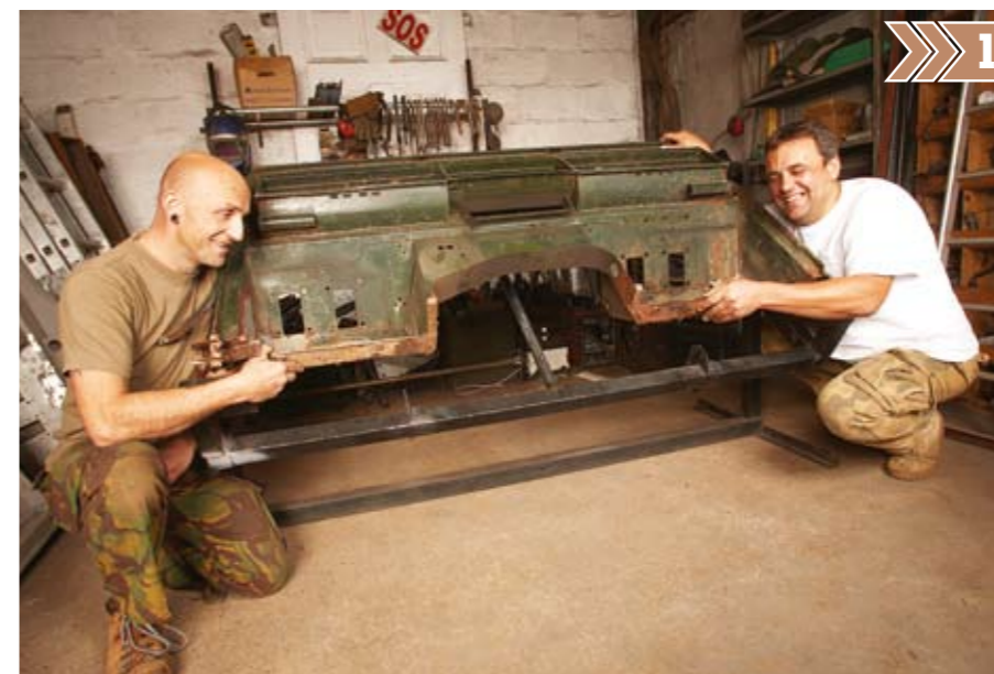
1 Kev and Lyn start by placing the bulkhead in their special jig and thoroughly inspecting it. ‘As long as you have the dash and the centre section’, says Lyn, ‘there’s enough to work with. Some need more work than others, but there aren’t many we have to write off completely.’
