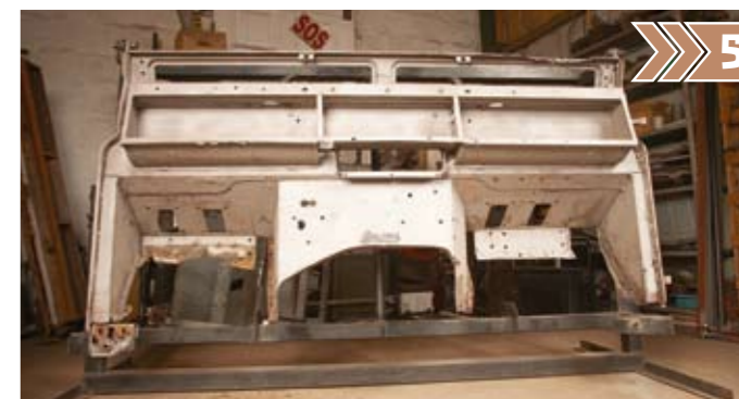
5 Many bulkheads will have years of layers of paint, possibly filler and all sorts of other nasties underneath the surface. The best approach is to get the bulkhead shotblasted, removing any loose rust and leaving clean metal to work with.
